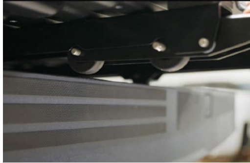
No Stop Rail drop - not enough extension past the edge of Tailgate.
